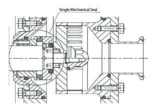
Slide the rotating part of the mechanical seal along the shaft facing the slot to the spindle until coming to the end of same. Then position the impeller on the shaft. Position the Seal and strongly tighten the nut by means of a spanner.
